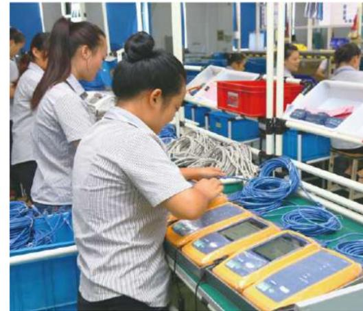
100% FLUKE Component Test for Patch Cord
